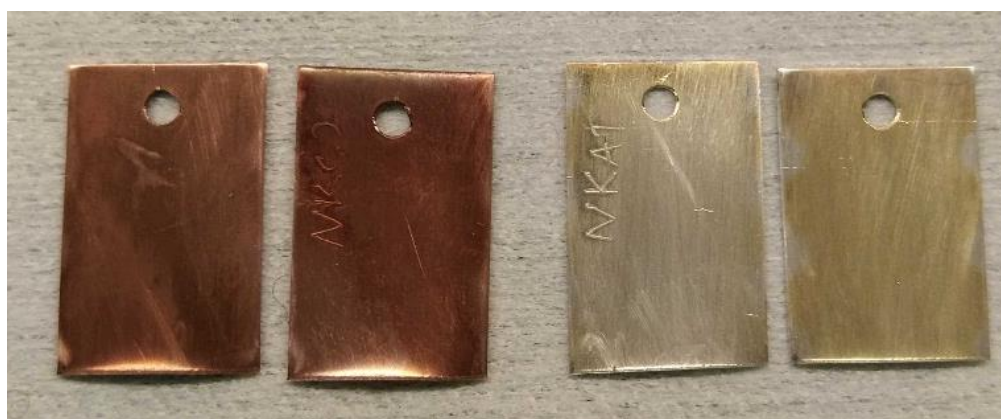
Figure 1. Coupons after the exposure. Copper coupons on left and silver coupons on right.
