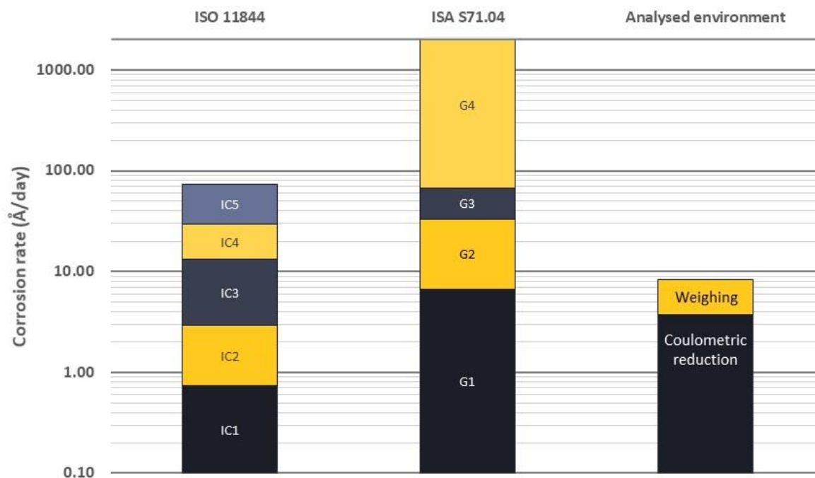
Figure 8. Comparison of silver corrosion rate to corrosion test standards.
